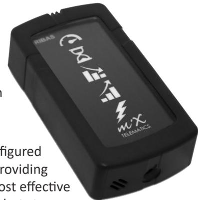
The device can be configured in a number of ways providing customers with the most effective method of delivering alerts to a driver. These options include an amber warning, notifying the driver that a parameter is close to exceeding the limit.
